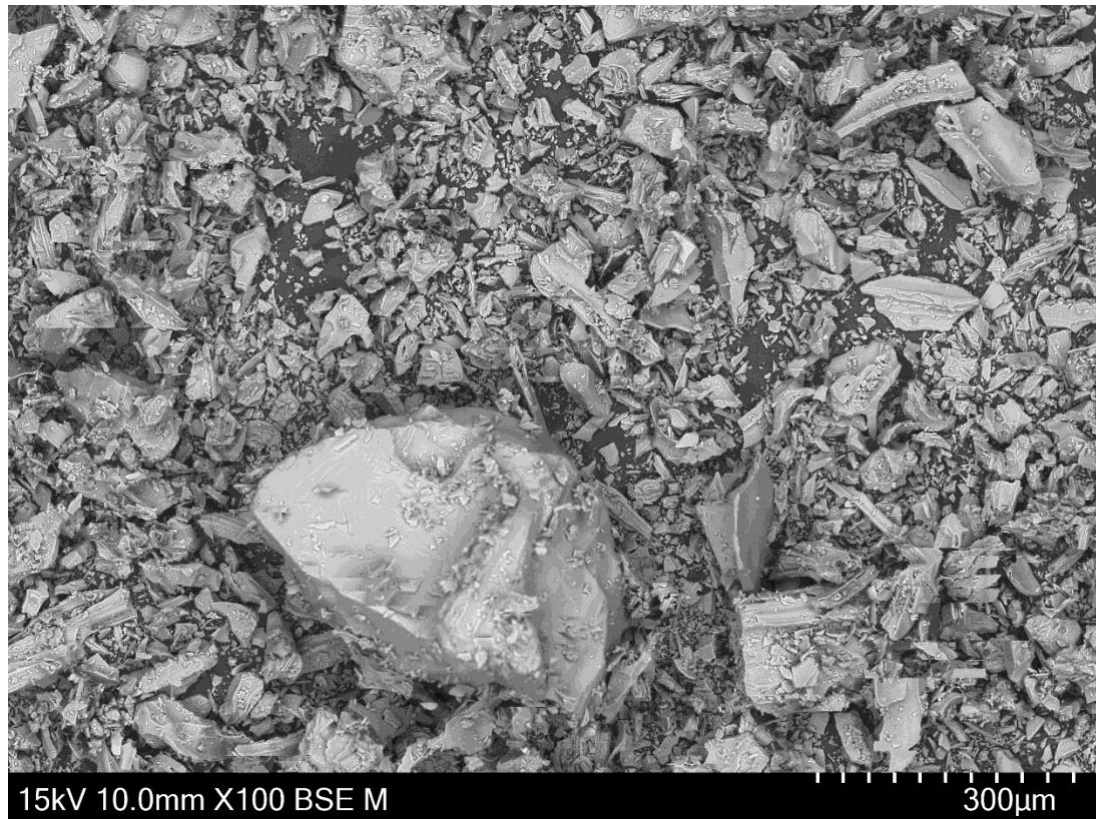
Figure 2.4. Scanning Electron Microscope image of Taupo 1 sample used in Chapters 5 and 6. Note the particle size, shape (angular, elongate and shard-like), and composition (glassy).
