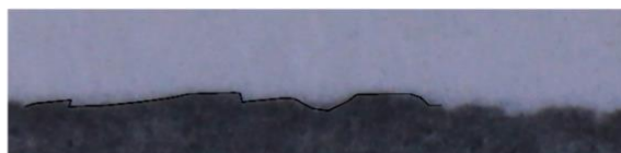
Sheared stepped deposit in Flume Run 3 (2.5% substrate, Section 4, Block C. ).
