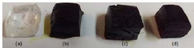
**Figure 3.** Photograph of 1 cm<sup>3</sup> of the hydrogels: (a) control hydrogel (**8**), (b) porphyrin hydrogel (**9**) with 4.0 mg of **5** (3.3 mM stock solution in PBS, pH=6.0) immobilized in it, (c) Cu(II)porphyrin hydrogel (**11**) with 4.1 mg of **7** (3.3 mM stock solution in PBS, pH=6.0) immobilized in it, (d) Pd(II) porphyrin hydrogel (**10**) with 4.4 mg of **6** (3.3 mM stock solution in PBS, pH=6.0) immobilized in it.
