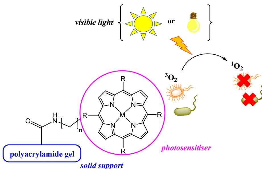
**Figure 1:** Schematic drawing of the photodynamic inactivation of microorganisms by singlet oxygen generated by the photosensitizer immobilized on a polyacrylamide support.
