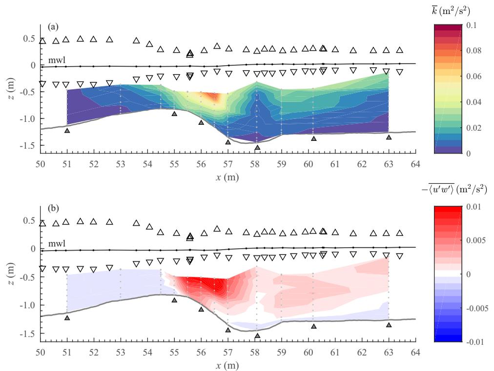
**Figure 4.** (a) Time-averaged turbulent kinetic energy; (b) time-averaged turbulent Reynolds stress. Open triangles at top mark maximum and minimum phase-averaged water surface. Grey dots indicate the outer-flow velocity measurement positions. Grey triangles at bottom mark the seven cross-shore locations for which detailed WBL velocities were measured.
