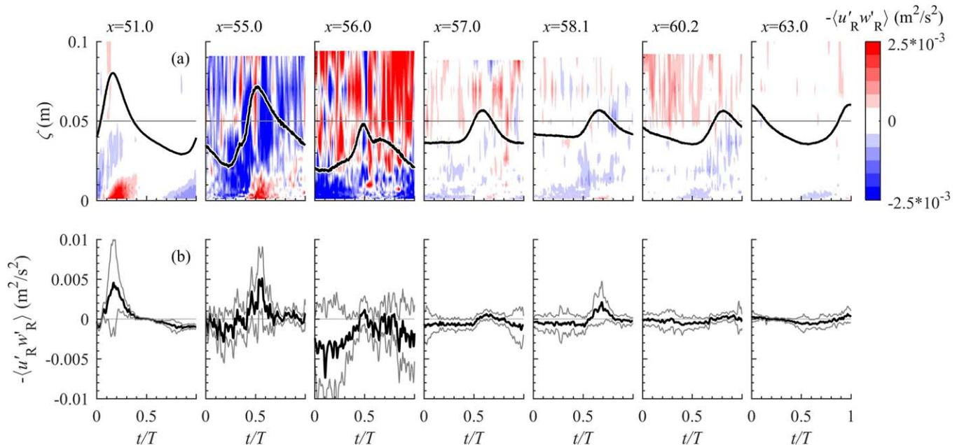
**Figure 7.** Phase-averaged turbulent Reynolds stress  $-\langle u'_R w'_R \rangle$ . (a) Depth-varying phase-dependent turbulent Reynolds stress (color contour), with the free-stream bed-parallel velocity  $\langle u_{R,\infty} \rangle$  (black line) for reference; (b) phase-averaged Reynolds stress at  $\zeta = 0.001$  m (black)  $\pm 1$  standard deviation (grey).
