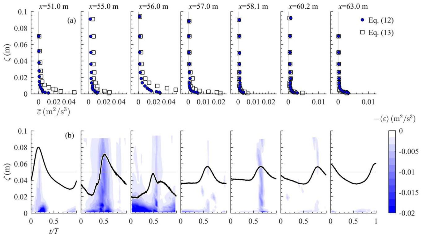
**Figure 9.** Turbulence dissipation rates. (a) Time-averaged dissipation, calculated through equation (12) (circles) and calculated through equation (13) (squares; note the different scales for the horizontal axes); (b) Phase-averaged dissipation as color contour, calculated through equation (12), with black line indicating free-stream velocity for reference.
