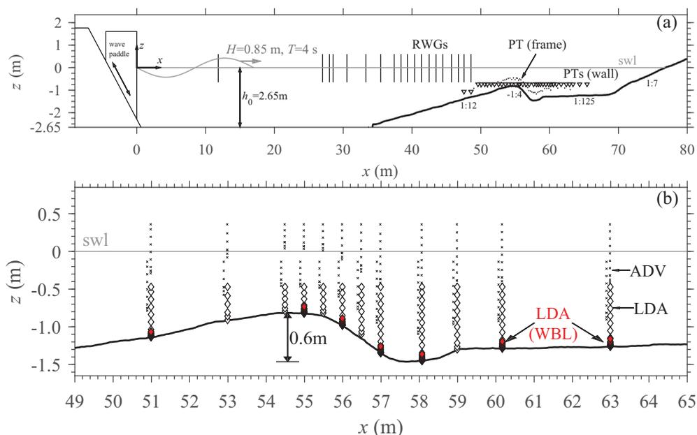
**Figure 1.** Experimental setup. (a) Locations of water surface elevation measurements by resistive wave gauges (RWGs; vertical black lines), side-wall-deployed pressure transducers (PTs wall; triangles), and mobile-frame PT (dots). (b) Close-up of barred test section, indicating velocity measurement locations by ADV (crosses), and LDA (diamonds). Red diamonds mark detailed near-bed measurements with LDA at seven cross-shore locations.
