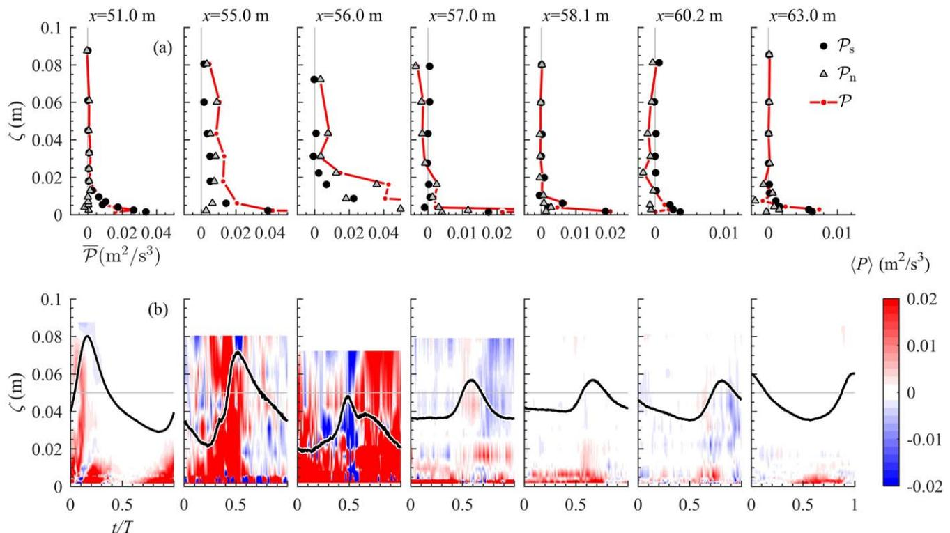
**Figure 8.** Turbulent production rates. (a) Time-averaged production, contribution by shear stresses (black diamond), contribution by normal stresses (grey triangle), and sum of both contributions (red dots and line; note the different scales for the horizontal axes); (b) Phase-averaged production  $\mathcal{P}$  as color contour, including free-stream bed-parallel velocity  $\langle u_{R,\infty} \rangle$  (black line) and  $\langle u_{R,\infty} \rangle = 0$  (grey line) for reference.
