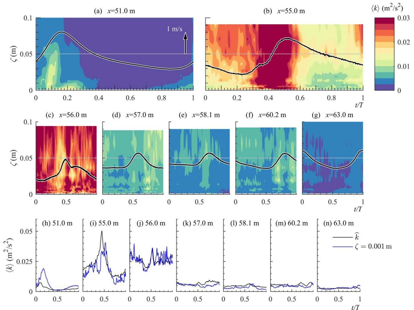
**Figure 5.** Time series of near-bed phase-averaged TKE. (a)–(g) depth-averaged phase-dependent turbulent kinetic energy  $\langle k \rangle$  (color contour), with the free-stream bed-parallel velocity  $\langle u_{R,\infty} \rangle$  (black line) for reference (arrow in (a) indicates velocity magnitude); (h)–(n)  $\langle k \rangle$  at  $\zeta = 0.001$  m (blue) and depth-averaged over near-bed control volume (black).
