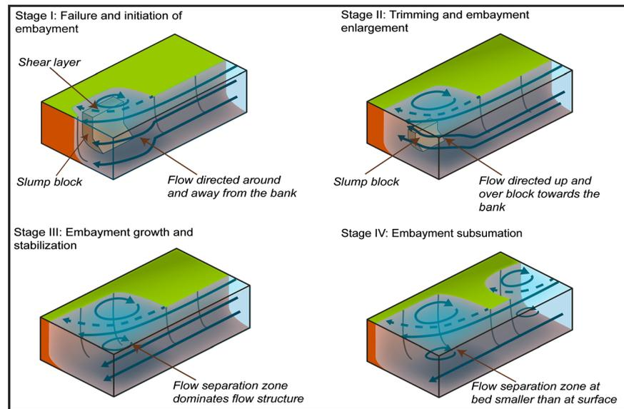
**Figure 4.** Conceptual model for the development of a bank embayment and the role that slump blocks play in diverting flow away from, and on to, the bank at different stages of embayment evolution. The black lines represent streamlines. The dashed lines represent the shear layer.
