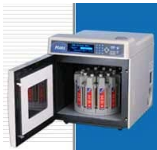
Fig. 1 Microwave oven (MARS, CEM) with the pressurized XP1500 digestion vessels used for experiment. Figure used with permission for reproduction obtained from Elsevier [License Number: 4197200736298].
