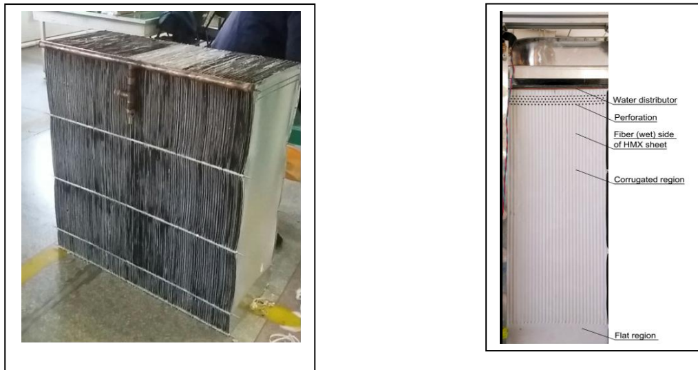
Fig. 2: Design drawings of the HMX.
