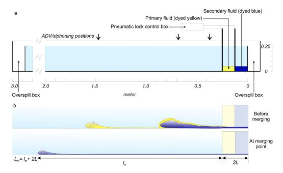
**Figure 1.** (a) Sketch of experimental setup (adapted from Ho et al., 2018). Note: (i) Three arrows sketched along the top of the flume indicate positions of Acoustic Doppler Velocimetry/siphoning instrumentation, (ii) two cameras were set up on a track fixed in front of the flume, (iii) initial flow height h = 0.05 m (see vertical scale bar). (b) Flow propagation model with lock length,  $L_m$ , merging length,  $I_m$ , and total merging length,  $L_m$ , highlighted.
