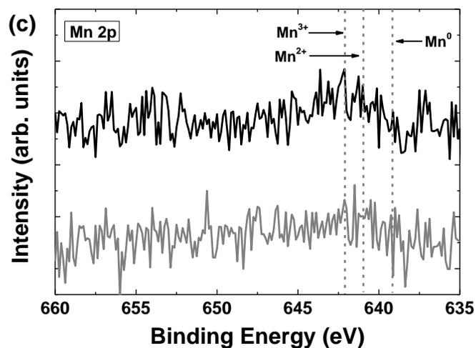
Figure S3. High-resolution XPS patterns for 3D S235-P steel before and after electrolysis for 2000 s: Fe 2p, P 2p, and Mn 2p.
