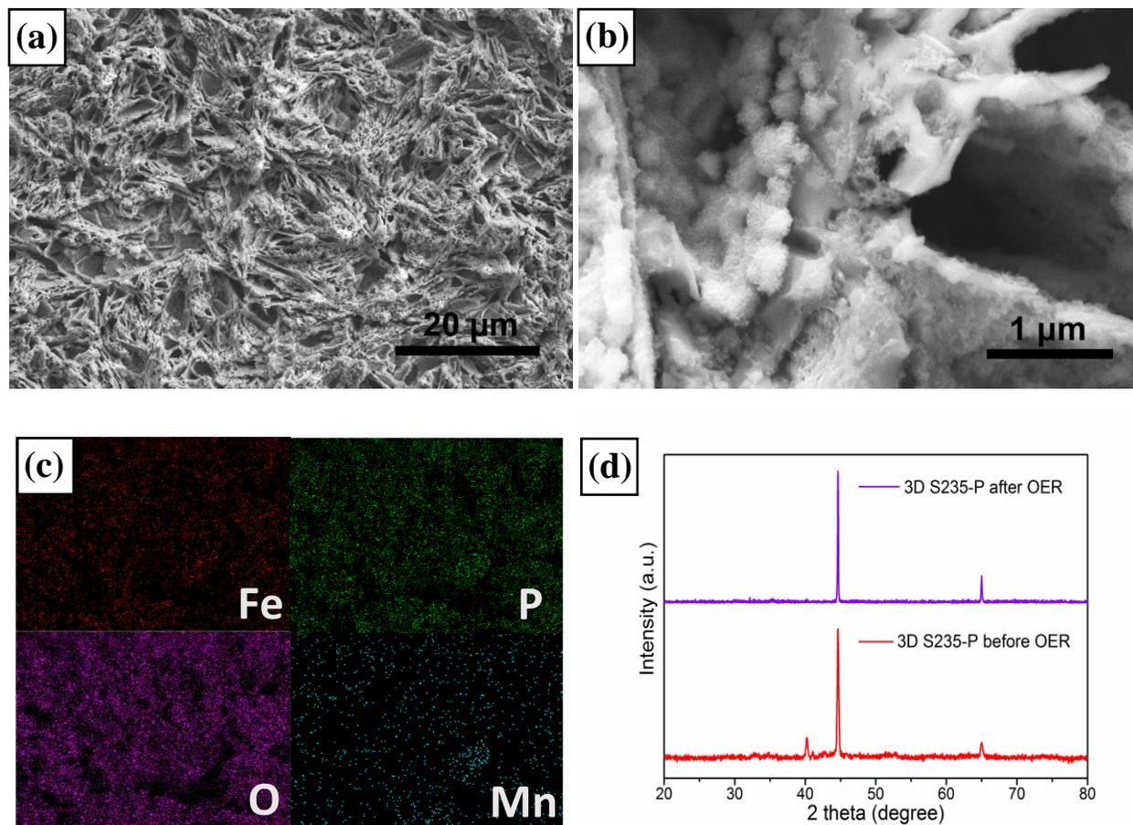
[Figure S5](#). SEM images (a, b) of the 3D S235-P steel after long-term chronopotentiometric measurement, (c) the corresponding elemental mapping images and (d) XRD patterns.
