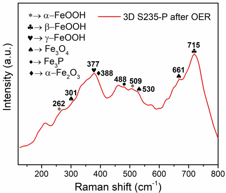
Figure S6. Raman spectrum of 3D S235-P steel after usage in OER testing.
