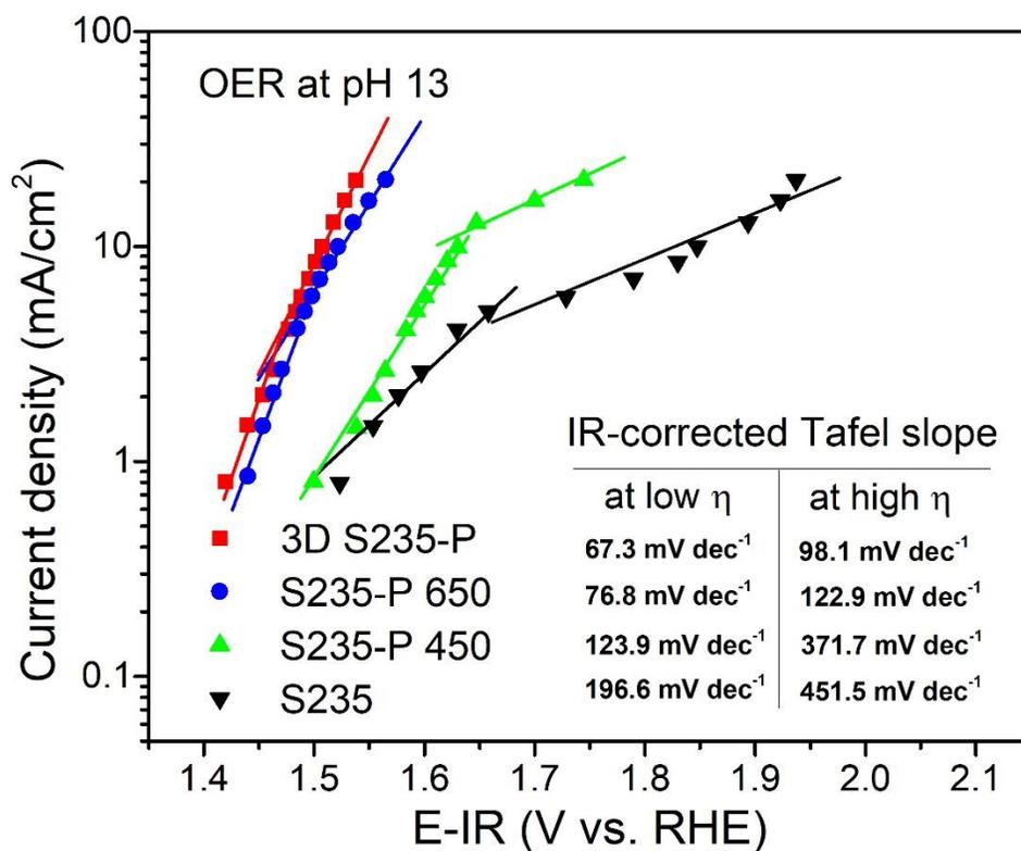
Figure S2. IR-corrected Tafel plots of 3D S235-P steel, S235-P-650 steel, S235-P-450 steel, and untreated S235 steel determined in 0.1 M KOH. Average voltage values for the Tafel plots were derived from 200 second chronopotentiometry scans at current densities 0.80, 1.48, 2.03, 2.67, 4.12, 4.98, 5.82, 7.07, 8.50, 9.98, 12.93, 16.36, and 20.34 mA cm<sup>-2</sup>. IR compensation was performed by taking in account the electrolyte resistance from EIS measurements (Figure 5).
