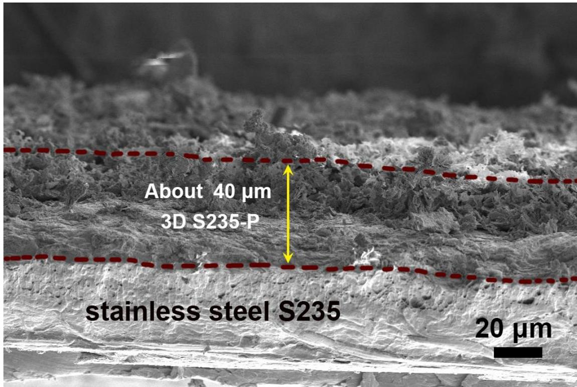
Figure S1. The cross-section SEM of 3D S235-P steel. The average phosphorized layer is about 40 μm.
