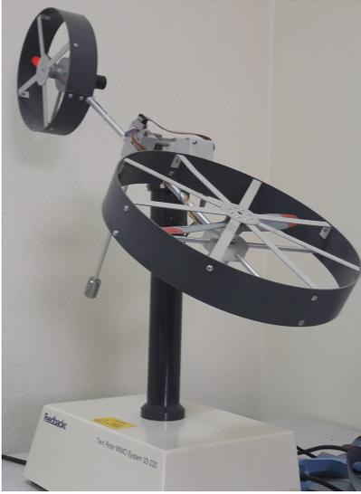
Fig. 1. Twin Rotor Multiple Input Multiple Output system
