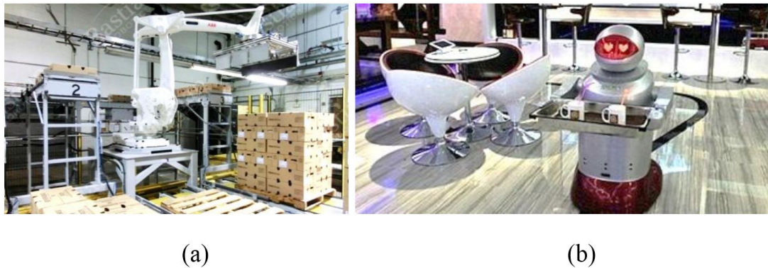
Figure 7. Robots in food industry: (a) IRB 660 for palletizing cartons; (b) Serving robot in China (Griffiths, 2014).
