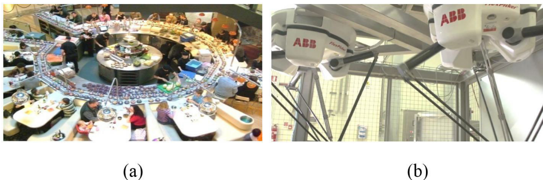
Figure 6. Productivity and workers' safety (a) Sushi serving concept through conveyor belt (DigPlanet, 2013); (b) Robots in operation in a completely isolated and properly fenced working area (ABB, 2016b).
