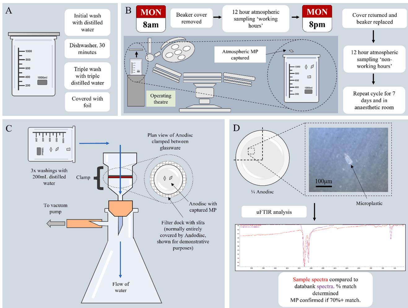
**Fig. 1.** Schematic of the methodology for detecting MPs in the surgical environment, (A) sampling beaker preparation, (B) atmospheric sampling, (C) sample filtration and MP capture onto Anodisc filter, (D) analysis of MP using  $\mu$ FTIR. Abbreviations: MP, microplastic;  $\mu$ FTIR, micro-Fourier-transform infrared spectroscopy.
