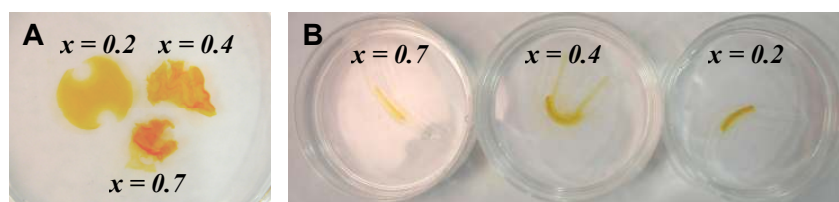
Figure 5.43: (A) Effect of concentration of ruthenium catalyst on the gel shape of poly(NIPAAm- co -Ru(bpy) 3 ) gels. The gel was polymerised in a perfusion chamber (diameter of 1.0 cm and thickness of 0.5 mm). (B) The swelling behaviour of the PNIPAAm/poly(NIPAAm- co -Ru(bpy) 3 ) bigel depending on the concentration of the Ru(bpy) 3 2+ moiety in the gel. x is the mole% of ruthenium catalyst Ru(bpy) 2 (mvbpy)(PF 6 ) 2 of the NIPA/Ru x /BIS1.3 gel.
