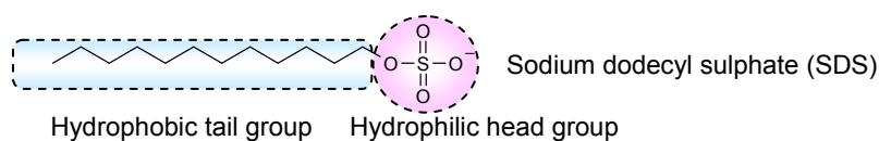
Figure 1.5: Schematic illustration of a typical surfactant molecule.
