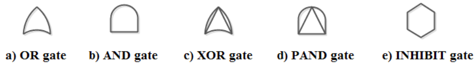
Figure 2—4. Fault tree symbols describing gates
