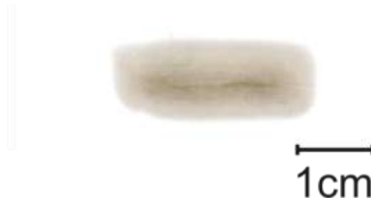
Figure 3-15 Transverse beam profile of the argon fluoride excimer laser obtained by irradiating thermal paper (fax paper) with 5 pulses of the raw beam. The beam can be seen to be approximately rectangular due to its highly multimode nature. In the vertical axis it is ~11mm in size and the irradiance distribution is roughly Gaussian. However, in the long, horizontal, axis it is ~27mm with uniform irradiance (the so-called “top-hat” distribution).
