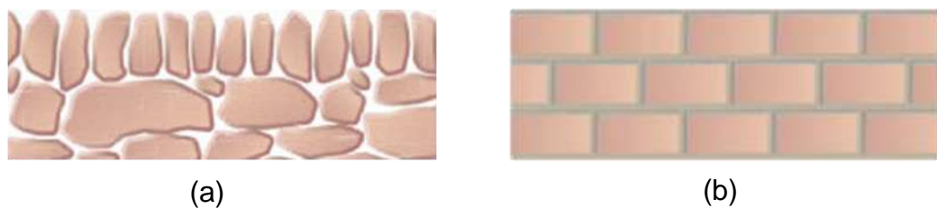
Figure 5-2 (a) skin like brick wall without enough mortar (b) Brick wall is strong and water tight with mortar [99].
