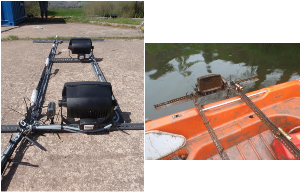
Figure 3.1 a) Left - Setup of camera arrays deployed in the lower Wye and Usk; b) Right - Camera and infrared light coated with algal growth.
