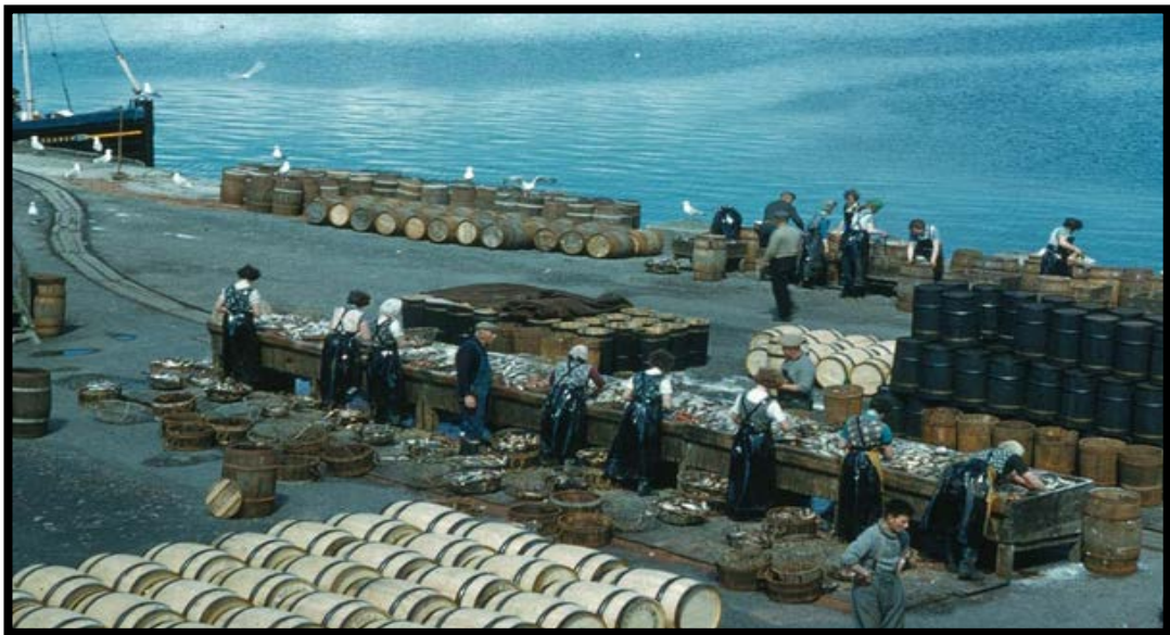
Figure 11. Gutting at J. and M. Shearer's herring curing station, Lerwick. Research LK 62 unloading at left. The tracks for the bogie can be clearly seen, as can the farlin in the centre. Source: SMAA, SL02775.
