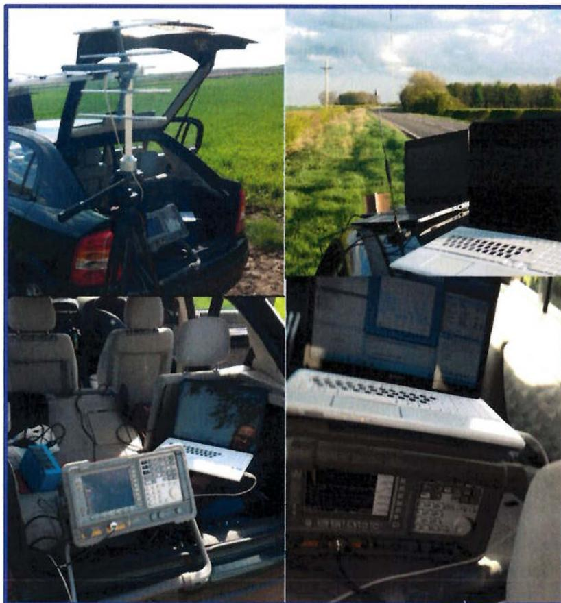
**Figure 5-2:** Measurement Equipment Employed in this Study: Antenna, Preamplifier and Spectrum Analyser at Rural Area (Humber region).
