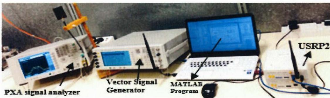
Figure 7-10: Test Bed for Experiments.
