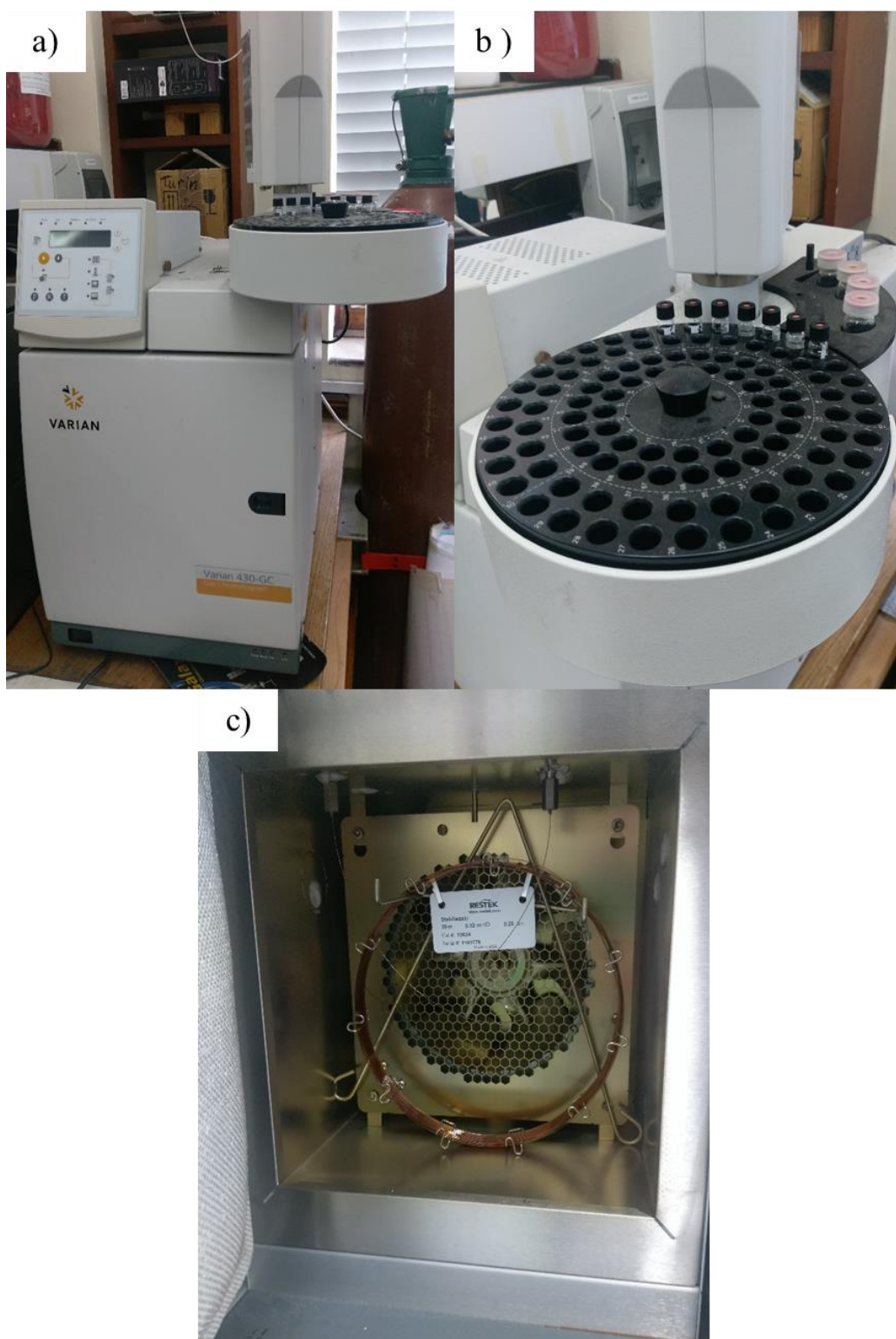
Figure 2. 22: a) The Varian 430 gas chromatograph that was used to complete the analysis. b) The Varian CP-8400 autosampler with sample vials placed in the carousel. c) The oven with Stabilwax® capillary column (Restek) attached to column hanger
