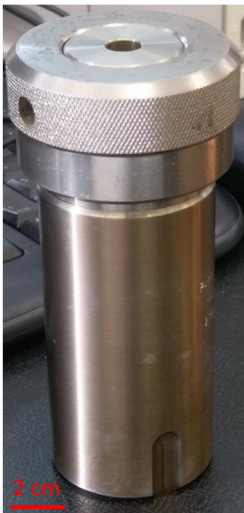
Figure 2. 2: Image of 50 mL Parr instrument company Teflon lined stainless steel autoclave reactor.
