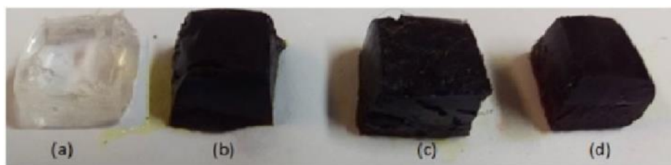
Figure 83 – Photograph of 1 cm 3 of the hydrogels: (a) control hydrogel (b) porphyrin hydrogel (69) with 4.0 mg of 69 (3.3 mM stock solution in PBS, pH=6.0) immobilised in it, (c) Cu(II)porphyrin hydrogel (71) with 4.1 mg of 71 (3.3 mmol L -1 M stock solution in PBS, pH=6.0) immobilised in it, (d) Pd(II) porphyrin hydrogel (70) with 4.4 mg of 71 (3.3 mM stock solution in PBS, pH=6.0) immobilised in it.
