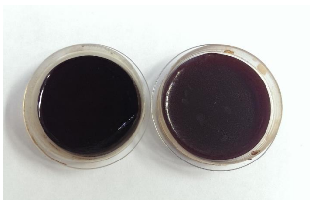
Figure 79 – Comparison of the gels formed using dioxane (left) and THF (right) as the solvent.
