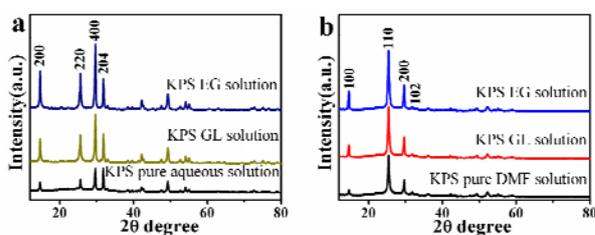
Fig. 2 XRD patterns of the whiskers prepared in different solutions at 90 °C. (a) aqueous solution; (b) DMF solution.
