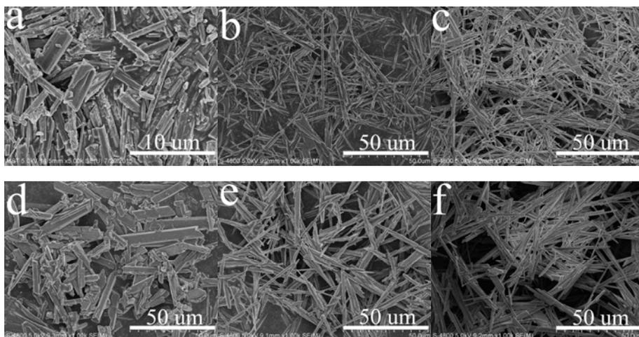
Fig. 1 SEM images of the samples prepared in different solutions at 90 °C. CaCl<sub>2</sub> aqueous solution and KPS aqueous solution (a), KPS EG solution (b) and KPS GL solution (c); CaCl<sub>2</sub> and KPS DMF solutions (d), KPS EG solution (e) and GL solution (f).
