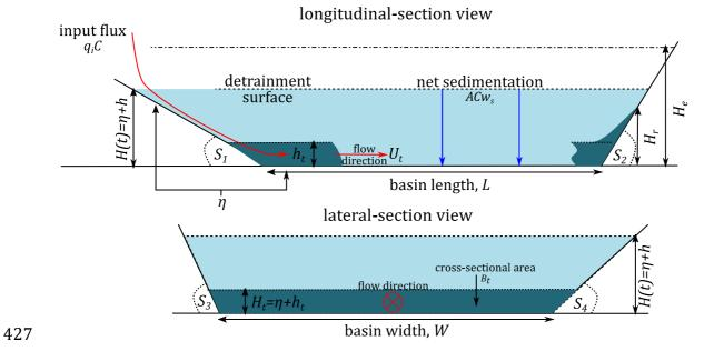
Figure 1. Schematic diagram of simplified model basin showing longitudinal and lateral-section views of the initial basin-floor flow and later ponded cloud inflation.
