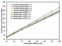
Fig. 13 Effect of Skutterudite thermoelectric leg length in SATEG and ATEG when  $\theta_1 = 6$  and  $\theta_2 = 2$ .
