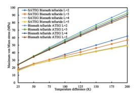
Fig. 12 Effect of Bismuth telluride thermoelectric leg length in SATEG and ATEG when  $\theta_1 = 6$  and  $\theta_2 = 2$ .
