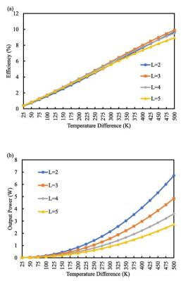
Fig. 10 Variation of Skutterudite ATEG leg length with (a) Efficiency and (b) Output power when  $\theta_1 = 3$ ,  $\theta_2 = 3$ , and  $R_L = 0.001 \Omega$ .
