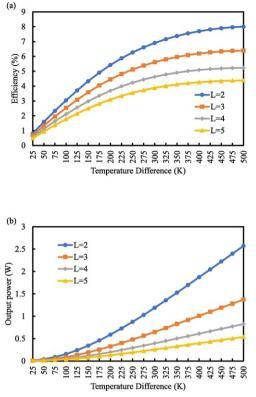
Fig. 11 Variation of SATEG leg length with (a) Efficiency and (b) Output power when  $\theta_1 = 3$ ,  $\theta_2 = 3$ , and  $R_L = 0.001 \Omega$ .
