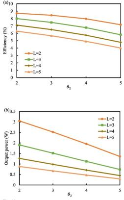
Fig. 14 Variation of leg angle with SATEG (a) efficiency and (b) output power when  $\theta = 8$ ,  $T_h = 623K$  and  $R_L = 0.001$ .
