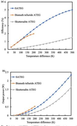
Fig. 7 Variation of SATEG and ATEG (a) efficiency and (b) output power with temperature difference when L=2,  $\theta_1=6$ ,  $\theta_2=2$  and  $R_L=0.01 \Omega$ .
