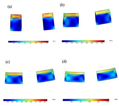
Fig. 16 Nephogram of the von Mises stress in Bismuth telluride material of the SATEG when L=2, Th = 623K,  $\theta_2 = 3$ , (a)  $\theta_1 = 3$ , (b)  $\theta_1 = 5$ , (c)  $\theta_1 = 7$  and (d)  $\theta_1 = 9$ .
