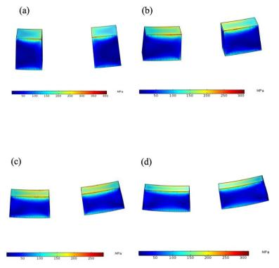
Fig. 17 Nephogram of the von Mises stress in Skutterudite material of the SATEG when L = 2,  $T_h = 623K$ ,  $\theta_2 = 3$ , (a)  $\theta_1 = 3$ , (b)  $\theta_1 = 5$ , (c)  $\theta_1 = 7$  and (d)  $\theta_1 = 9$ .
