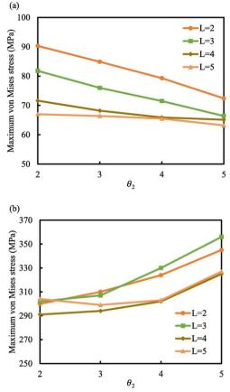
Fig. 15 Variation of leg angle with maximum von Mises stress in (a) Bismuth telluride and (b) Skutterudite materials of the SATEG when  $\theta$  = 8 and  $T_h$  = 623 K.
