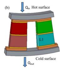
Fig. 1 SATEG geometry; (a) schematic diagram and (b) three-dimensional view.
