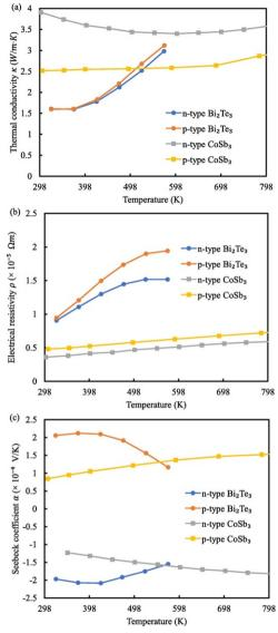
Fig. 4 Temperature dependent thermoelectric properties [47]: (a) thermal conductivity, (b) electrical resistivity, (c) Seebeck coefficient.
