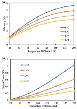
Fig. 9 Variation of Bismuth telluride ATEG leg length with (a) Efficiency and (b) Output power when  $\theta_1$  = 3,  $\theta_2$  = 3, and  $R_I = 0.001 \Omega$ .
