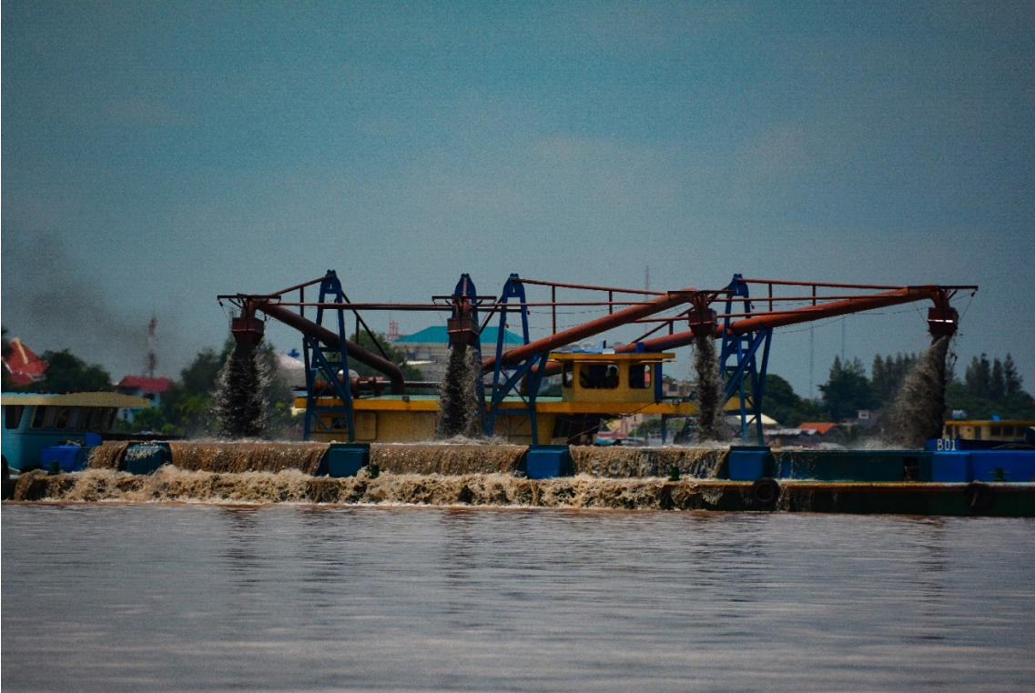
Suction dredgers mining sand in the Mekong River near Phnom Penh, Cambodia
