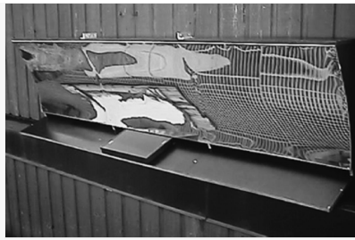
Photograph of a ST5 photovoltaic module from Siemens in a concentrating reflector system. An identical reference module was mounted in the vertical plane of the aperture [66].
