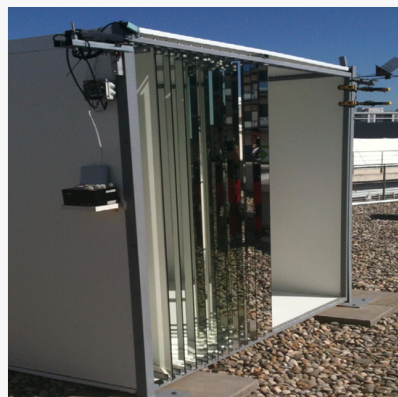
The reflectors facade: during the installation of the concentrating PV façade at the Applied Energy Research Centre (CREA) at the University of Lleida (Spain). The tracking system is noticed on the left [40].
