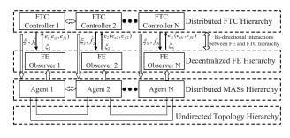
Fig. 1. Hierarchical structure-based design with bi-directional interactions between the FE and FTC hierarchy.
