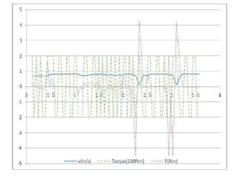
Fig. 12. (Colour online) Robot control and velocity (driving force  $F_d$ : dot; steering torque  $\tau$ : dashed; velocity v: solid).
