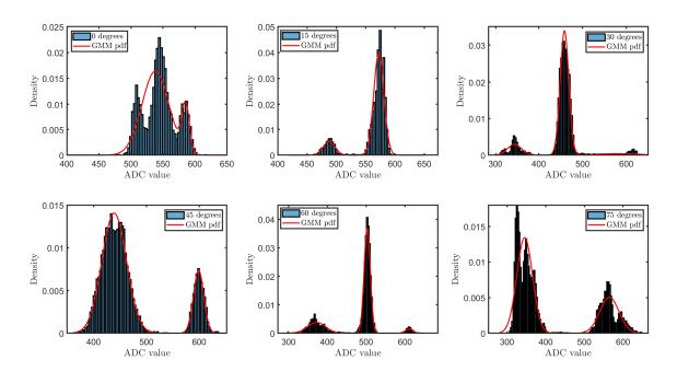
Fig. 10. Histogram plots and respective mixed gaussian distribution fits of the sensor's output at (a)  $0^{\circ}$  (b)  $15^{\circ}$  (c)  $30^{\circ}$  (d)  $45^{\circ}$  (e)  $60^{\circ}$  (f)  $75^{\circ}$
