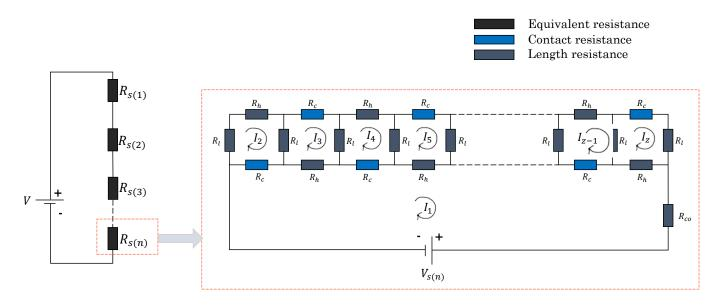
Fig. 2. Circuit model of the weft knit sensor. (Z - 1) is the number of wales in the sensor.
