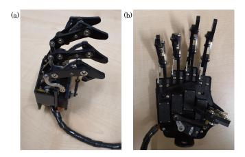
Fig. 5. Robotic hand used for glove evaluation. (a) Side view (b) Front view illustrating its motors.
