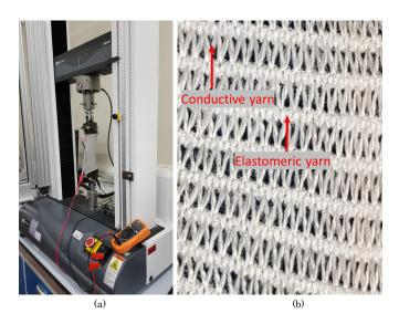
Fig. 3. (a) Experimental setup with Instron 3369 and Multimeter. (b) Image of sensor's loop configuration.
