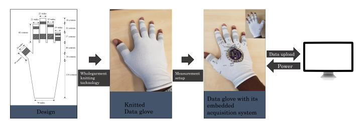
Fig. 4. Block diagram illustrating the design and implementation of the weft knit Data glove.
