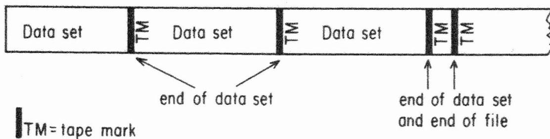
Figure 5. Multiple data sets on an IBM unlabelled tape
