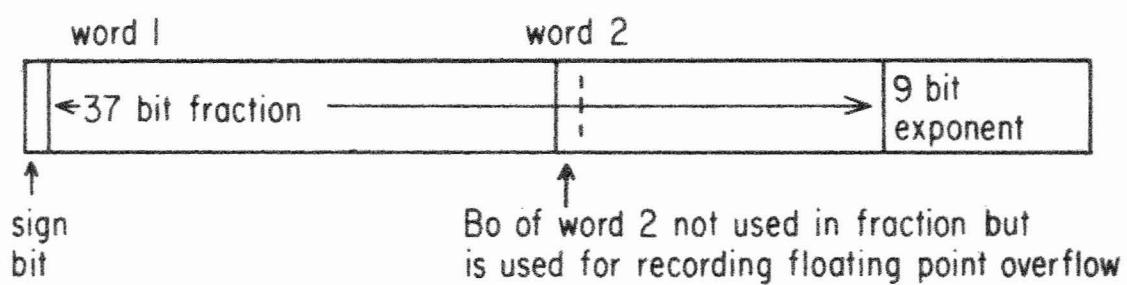
Figure 3. Internal representation of floating point numbers
