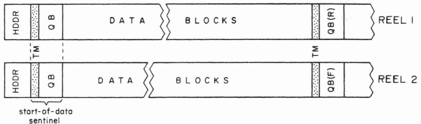
B) IBM 360 (all blocks are separated by interblock gaps)
