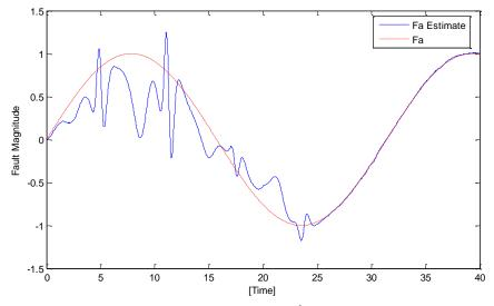
Figure 4: Fault signal  $f_a$  and fault estimate  $\widehat{f}_a$  with AFTC activated at 20s
