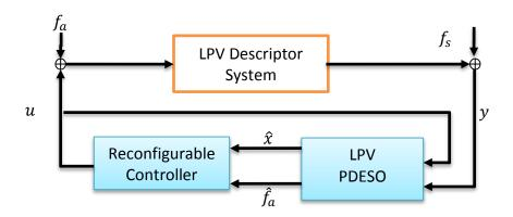
Figure 1: The structure of AFTC for LPV descriptor systems with PDESO
