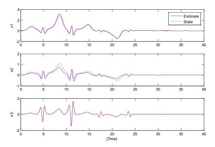
Figure 5: States & their estimates before and after the AFTC activated at 20s
