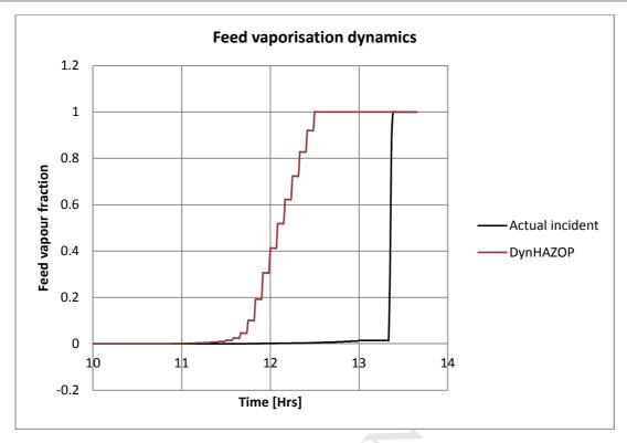
Figure 7: Dynamic HAZOP feed vapourisation dynamics
