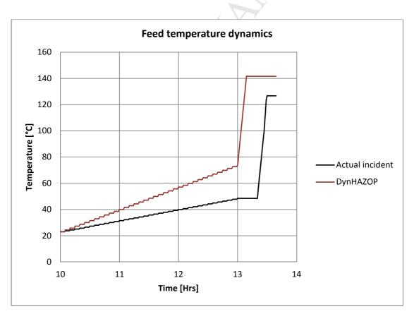
Figure 6: Dynamic HAZOP feed temperature dynamics
