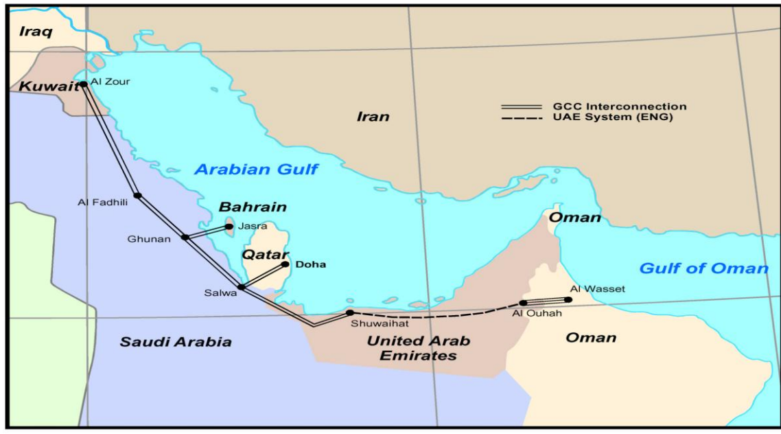
Figure 11 GCC Interconnection Grid
