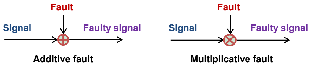
Figure 2-1 Additive and multiplicative faults
