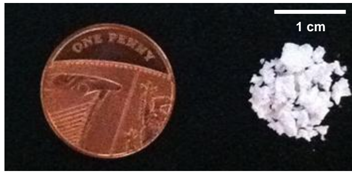
Figure 3-3 Photograph of silica monolith prepared from TMOS + 1 M nitric acid + PEO using microwave heating at 180-260 °C for 10 min and 300 W.
