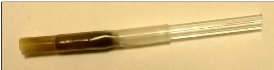
Figure 4-13 Silica monolithic column using microwave heating for 50 min at 80 °C during C 18 surface modification.
