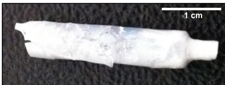
Figure 3-6 Photograph of silica monolith prepared from TMOS + 1M nitric acid + PEO using microwave heating with this condition 1 min at 10 W then 1 min at 20 W then 1 min at 40 W then 1 min at 80 W then 1 min at 160 W.
