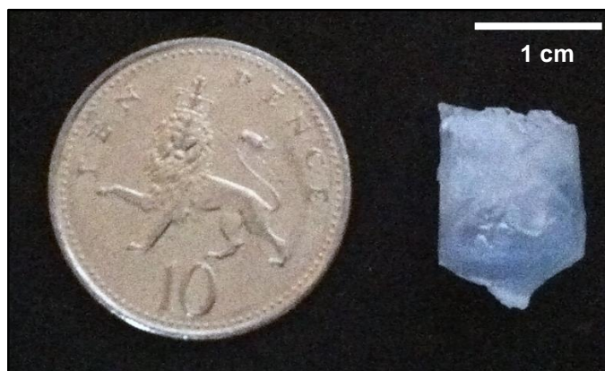
Figure 3-5 Photograph of silica monolith prepared from TMOS + 1 M nitric acid + PEO using microwave heating at 40 °C for 30 min and 50 W.
