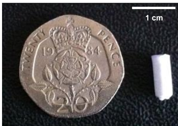
Figure 3-7 Photograph of silica monolith prepared from TMOS + 0.02 M acetic acid + PEO using microwave heating with this condition 1 min at 10 W then 1 min at 20 W then 1 min at 40 W then 1 min at 80 W then 1 min at 160 W.
