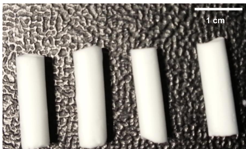
Figure 3-10 Photograph of (TMOS + PEO + 0.02 M acetic acid) monolith obtained using microwave heating at this condition 2 min at 10 W then 2 min at 20 W then 2 min at 40 W then 2min at 80 W then 2 min at 160 W then 1 min at 300 W.
