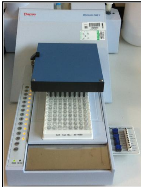
Figure 4-20 Thermo Labsystems Wellwash 4 MK 2 Microplate Washer for 96-Well Plates Performing Washes
