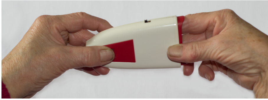
Figure 6.2: The EIMO device being held in use. The left hand thumb presses against the outside ECG pad. The right hand first and second fingers touch the inside ECG pad and the two PPG sensors in the insert (Munnock & Jiang, 2015). This normally takes place when the device is in a relaxed position for the user.
