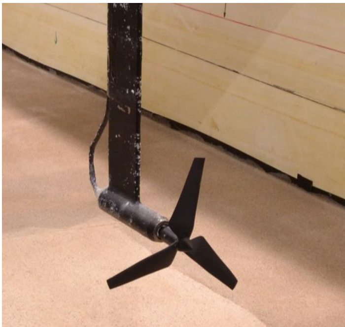
Figure 1.3: Model three-bladed horizontal axis tidal stream turbine used during experiments.
