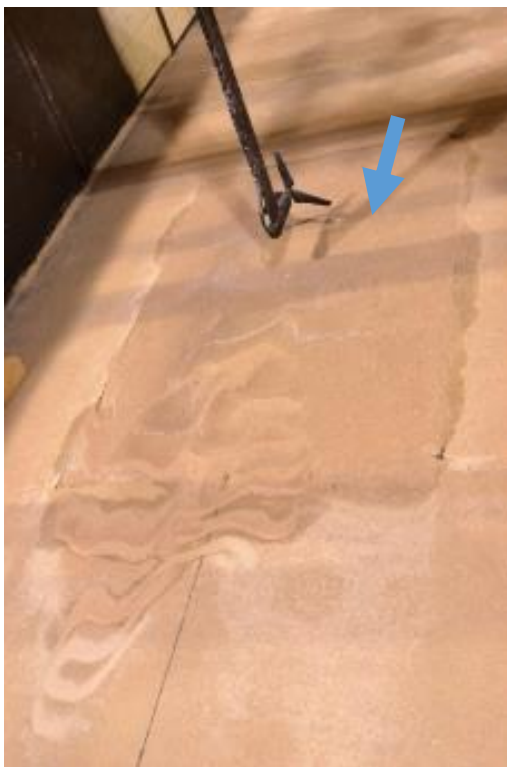
Figure 5.20: Image of scour in the mobile bed inset when the rotor was at 120mm above the bed. The actual extent and degree of the scour and sediment transport were not quantified. Blue arrow shows flow direction.
