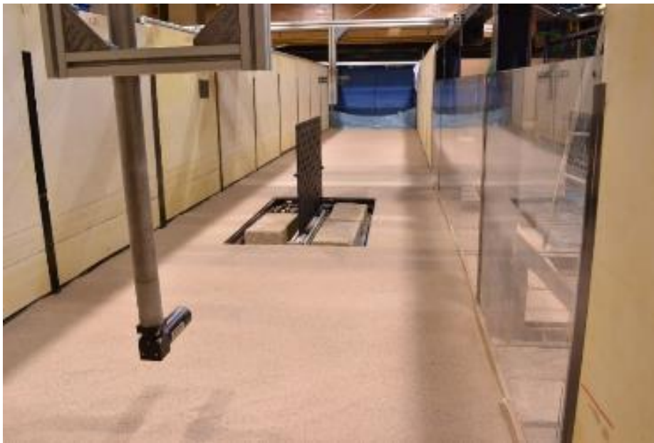
Figure 3.14: Calibration target within the channel. The PIV optic can be seen in the lower of the image, with the multi-level target visible upstream.
