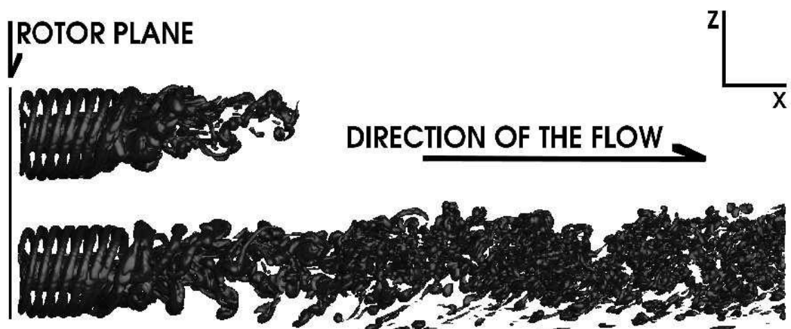
Figure 2.8: Side view of the vorticity field of a turbine wake. The top image shows the early stages of the wake development (after 42 seconds) and the bottom image shows the wake development after 189 seconds (Vybulkova et al. , 2013).
