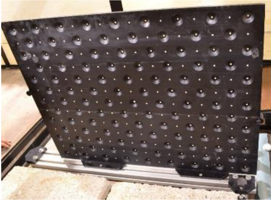
Figure 3.13: Multi-level target used to obtain a 3D calibration for the PIV system.
