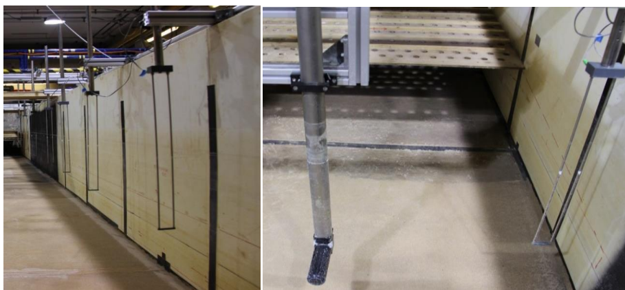
Figure 3.19: Left image: Wave gauges situated along the right hand side of the channel. Right image: Close up of furthest downstream wave gauge, positioned close to the laser optic.
