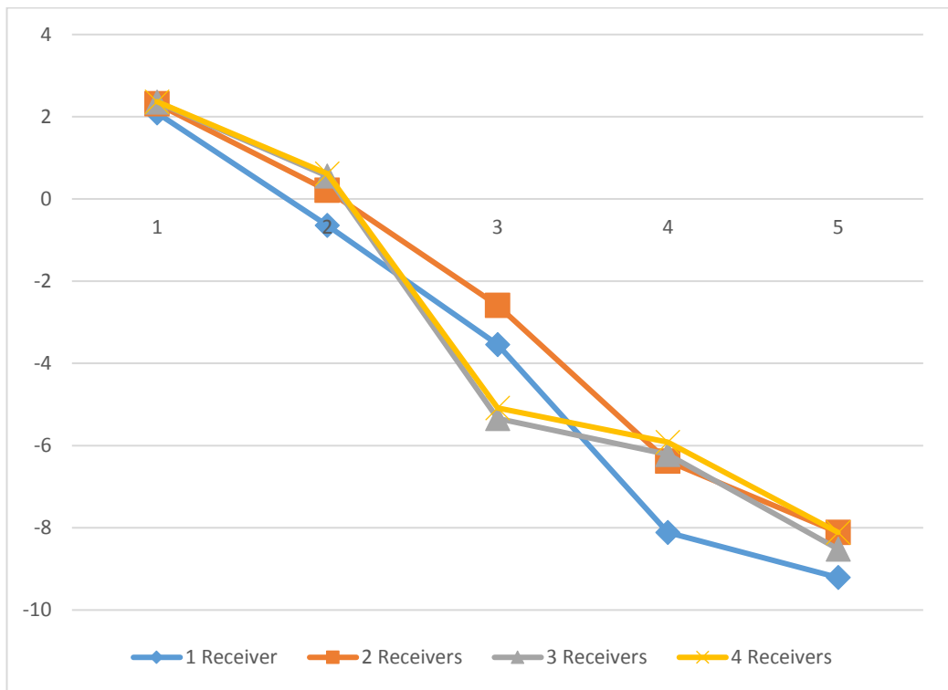
Figure 3.2b Singular values for linear dipole antenna system with 1-4 RXs for a mine placed under an antenna
