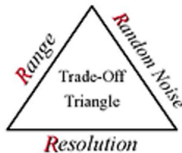
Figure 43: The ADCP ‘trade-off triangle’ between Range, Random Noise and Resolution (Teledyne, 2011).
