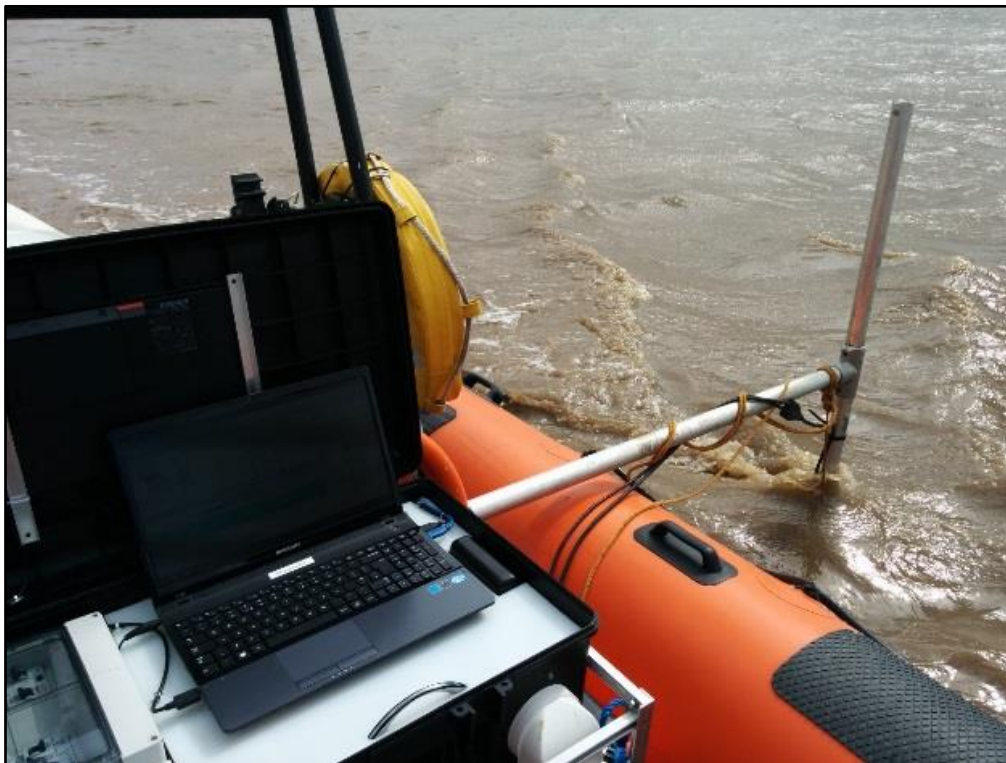
Figure 61: Photograph of vessel-mounted ADCP setup in the field.
