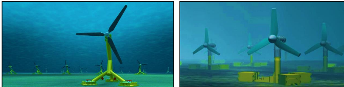
Figure 3: Bed-mounted turbines; Atlantis' AR1500 and Andritz Hydro Hammerfest's HS 1000 (ATC, 2016; ScottishEnergyNews, 2016).
