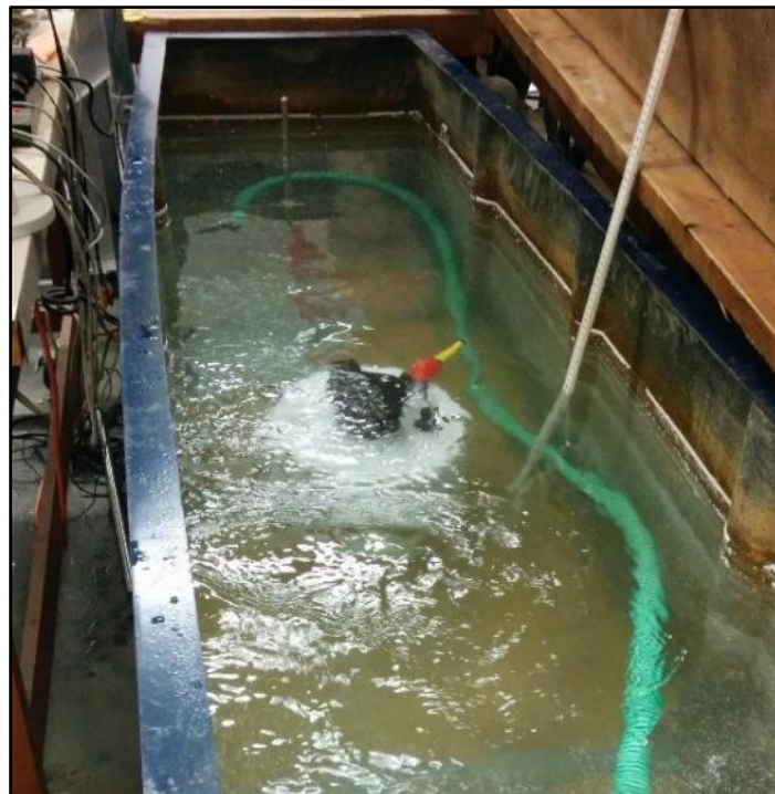
Figure 54: Testing the flow direction output of MIDAS DWR in uni-directional flume.
