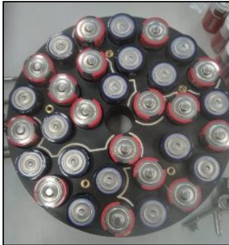
Figure 52: Battery configuration of the Valeport MIDAS DWR using 32 1.5 V alkaline D-cells.
