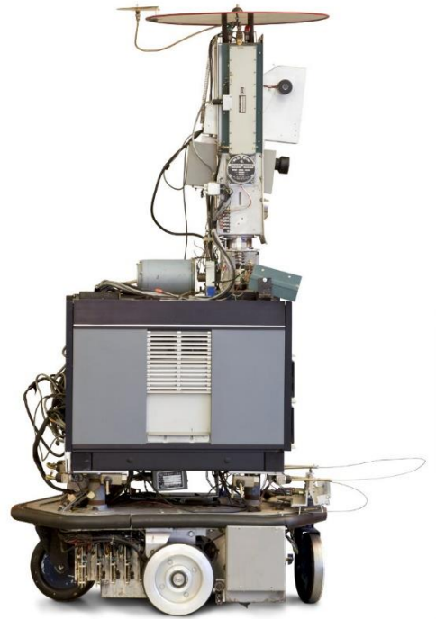
Figure 2-2 - Shakey the robot. Shakey the robot (Fikes & Nilsson 1971) was one of the first autonomous robots that used a deliberative control architecture.
