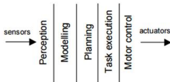
Figure 2-1 - Hierarchical decomposition of a mobile robot control system.
