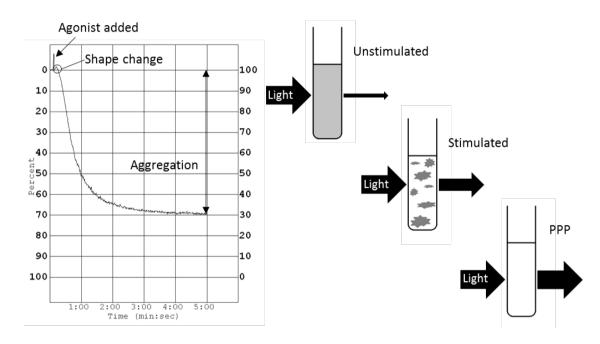
Figure 2. 3: Principles of Light Transmission Aggregometry
