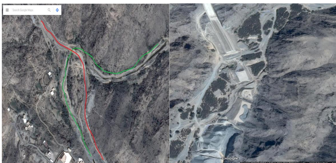
Figure 2.8. Left: Al-Janabeen Wadi (green line) intersected by a road (red line). Right: Wadi Thhrad upstream of Thhrad reservoir as an example of digging in the mountains and wadis for road construction.
