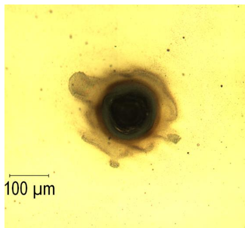
Figure 7.2: A typical irradiated spot of SiC by \text{CO}_2 laser at 150 \mu\text{s} and 500 pulses repetition rate. The attenuator set the applied power to 8.5 W.
