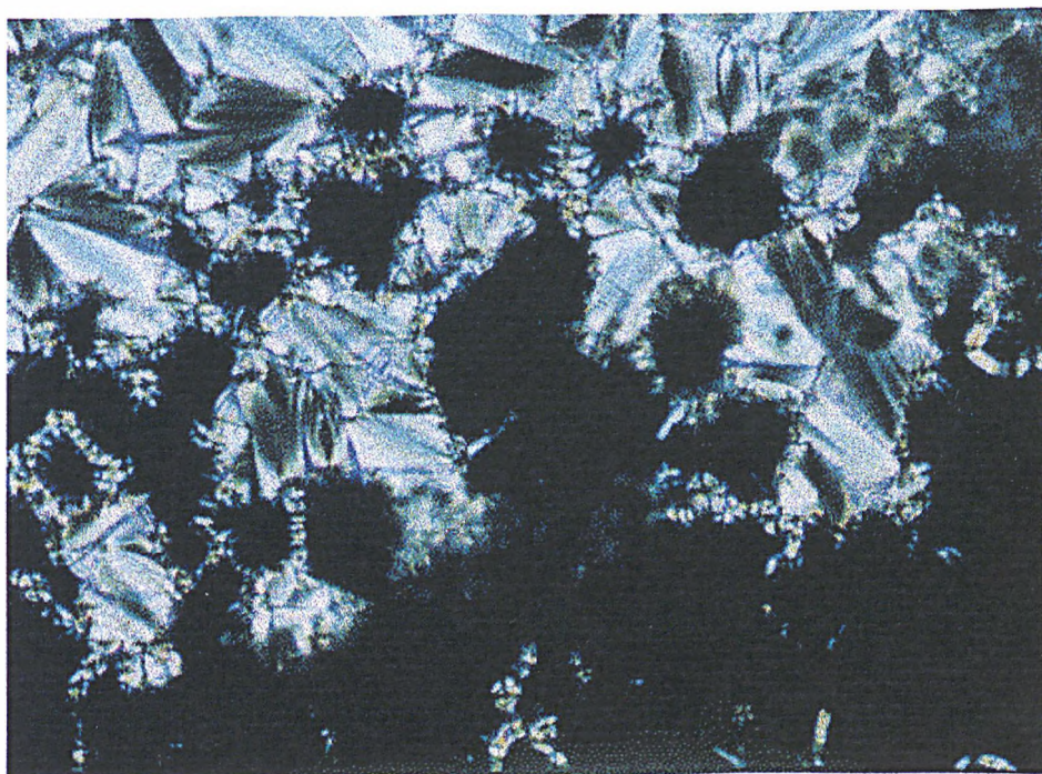
Plate 8 The SmI* phase of ( R )-MHPOBC at 55 °C
