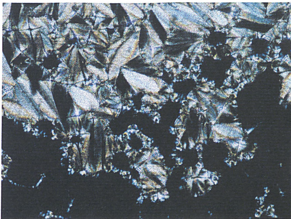
Plate 3 The SmC* phase of ( R )-MHPOBC at 119 °C
