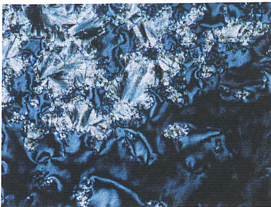
Plate 10 The SmC phase of (±)-MHPOBC at 120.9 °C
