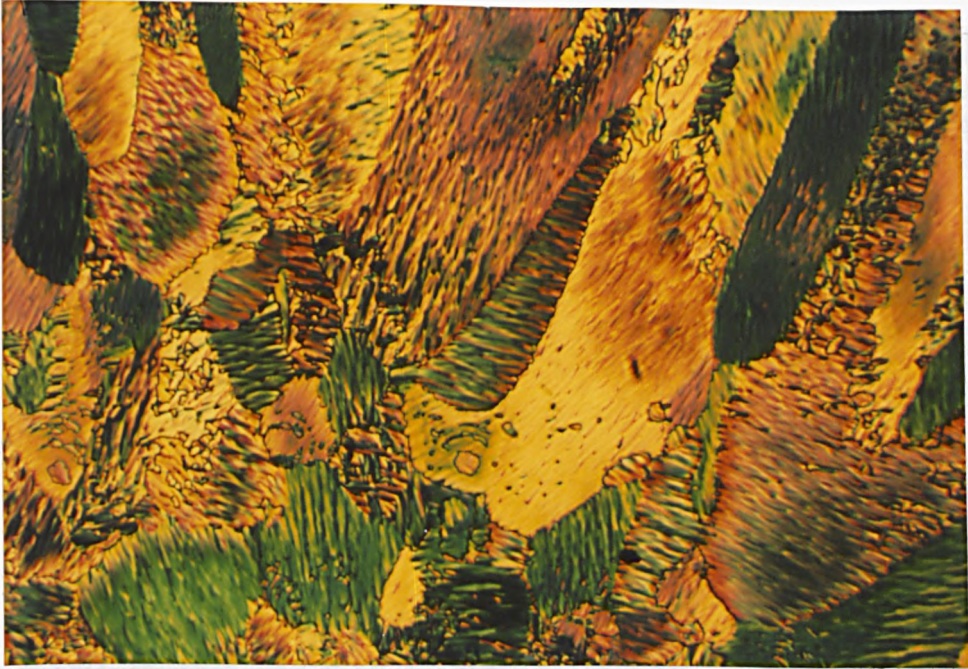
The Focal Conic Fan Texture of the Cholesteric Mesophase
