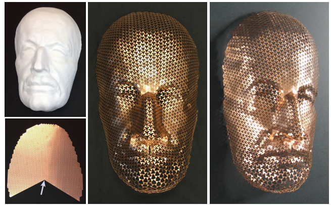
Figure 15: Fabrication of the Max Planck model. Top left: 3D printed reference model used for geometric guidance; Bottom left: flat, undeformed perforated copper sheet. The purple arrow indicates the singular vertex located at the tip of the nose; Middle, Right: two photographs of the final model.
