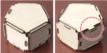
Figure 13: Our method can generate steady interlocking assembly (left) and avoid non-steady connections due to tolerance (right).
