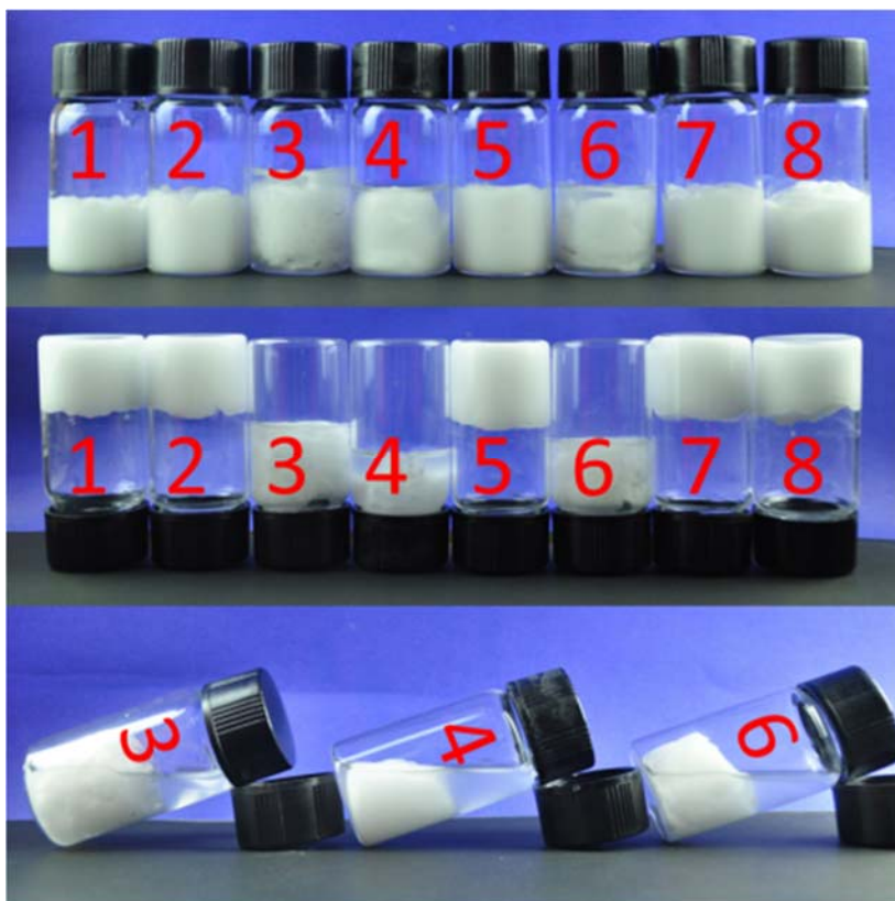
Figure S1. Digital photos of W/O Pickering emulsions with different formulations 30 min after emulsification: (1) P 6 S 2.5 -70, (2) P 6 S 2.5 -75, (3) P 6 S 2.5 -80, (4) P 6 S 2.0 -75, (5) P 6 S 3.0 -75, (6) P 7 S 2.5 -75, (7) P 5 S 2.5 -75, (8) P 4 S 2.5 -75.
